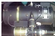
Diesel powered heater
