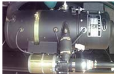
Diesel powered heater
