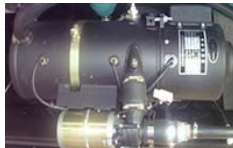
Diesel powered heater
