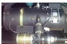
Diesel powered heater
