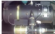
Diesel powered heater
